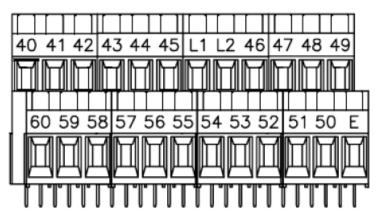
The fuel select switch connects to terminals 45, 49 and 53.
