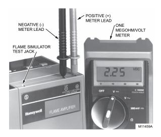
Fig. 4. Flame signal measurement with meter.
