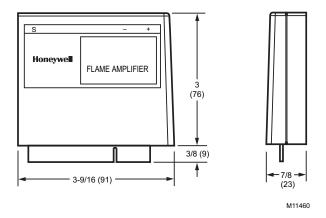
Fig. 1. Flame amplifier dimensions in in. (mm).
