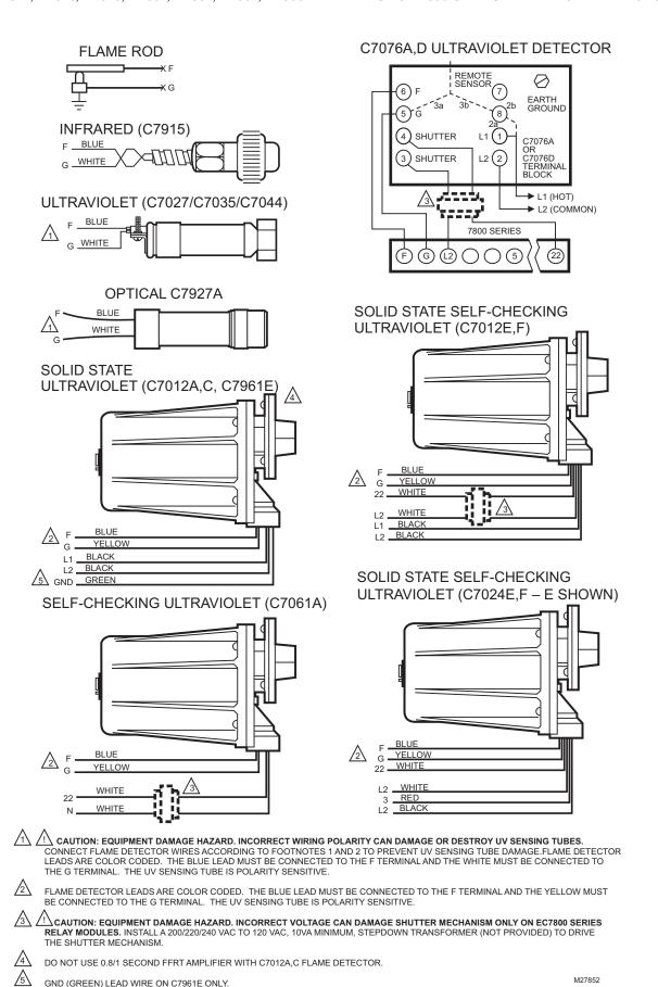
Fig. 3. Flame detector wiring.
