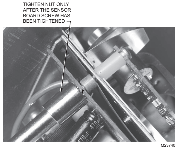
Fig. 8. Tighten circuit board retaining nut.
